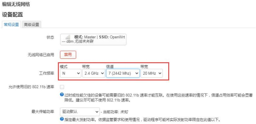
7) Then in **Interface Configuration ->General Settings**, set the mode to **Access Point AP**, **ESSID** (Wireless Network Name) to **OpenWrt**, and network to **wan**
