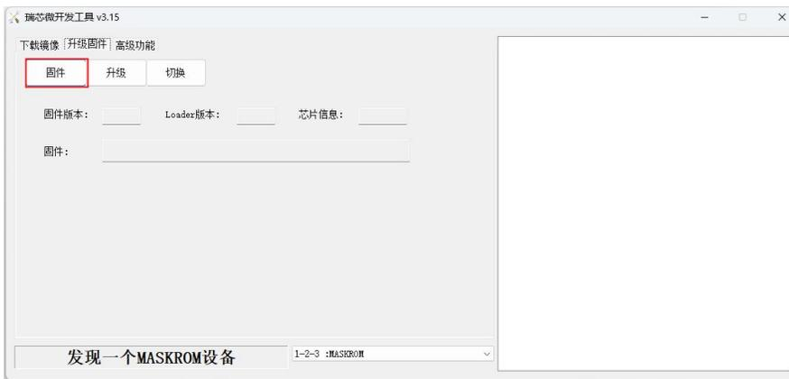
h. Finally, click the "Upgrade" button to start burning. The log of the burning process is shown in the figure below. After the burning is completed, the Android system will automatically start.
