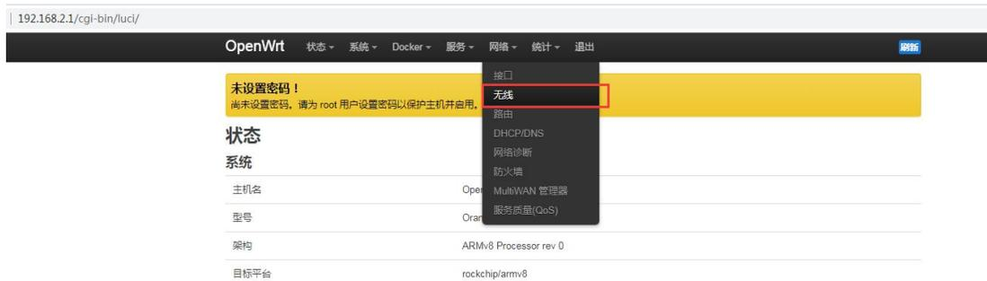
3) The default wireless configuration of OpenWRT system is **Master** mode. For the convenience of the next operation, we will remove the default wireless connection.
