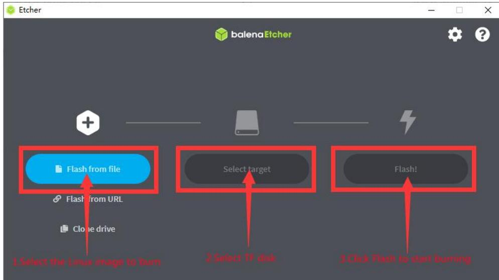
10) The interface displayed during the process of burning a Linux image with balenaEtcher is shown in the following figure. In addition, the progress bar displays purple to indicate that the Linux image is being burned to the TF card.
