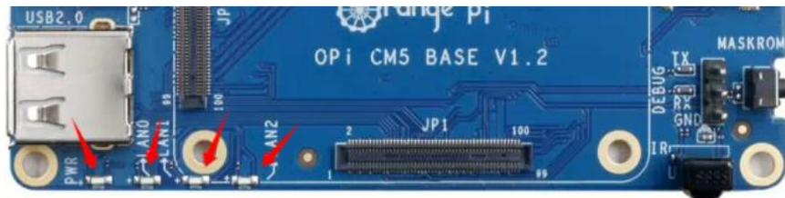
2) As long as the development board is powered on, the red LED light will be always on. This is controlled by hardware and cannot be turned off by software. The red LED light can be used to determine whether the power of the development board has been turned on normally.
