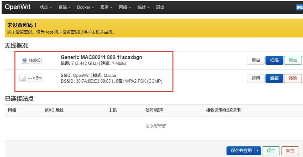
12) Then use your phone or computer to search for the corresponding WiFi SSID for connection. After successful connection, as shown in the following figure
