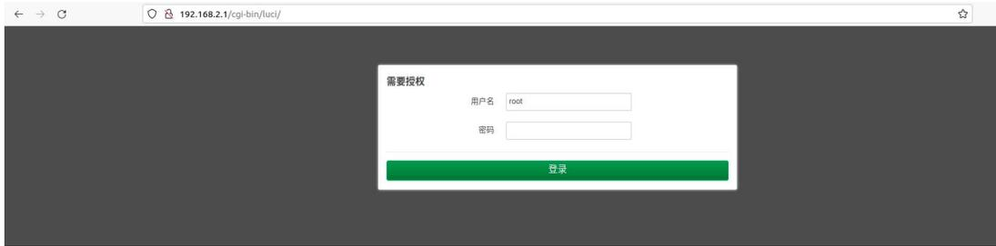
4) **OpenWrt 系统默认是没有设置密码的，所以 The OpenWrt system does not have a password set by default**, so simply click the **login** button. After successful login, the interface will display as shown in the following figure
