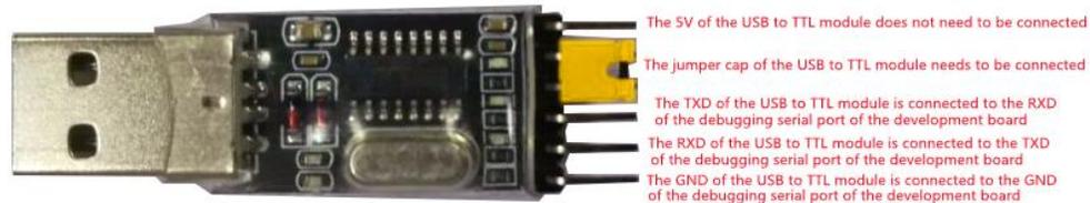
2) The corresponding relationship between the GND, RX and TX pins of the debug serial port of the baseboard is shown in the figure below:
